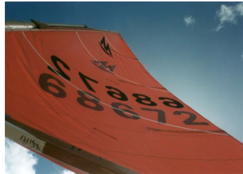
Figure 5: Sail with camber stripes.
